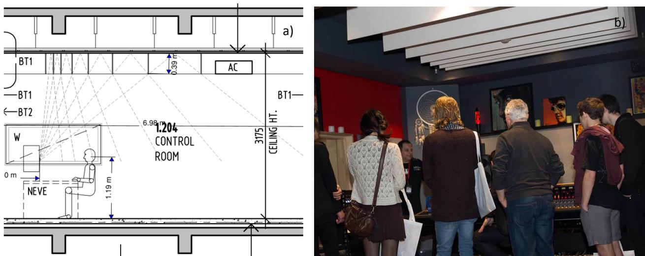
Figure 5: Control Room Ceiling First Reflection Treatment. a) Room section showing loudspeaker source and ceiling baffling. b) View of ceiling baffles in control room.
