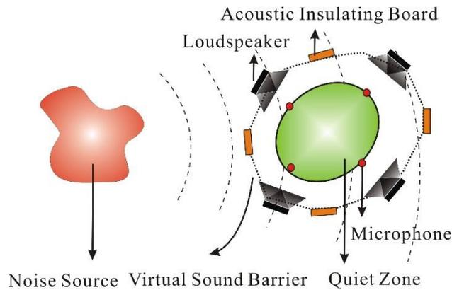
Figure 6: Schematic drawing of a partition hybrid VSB system
