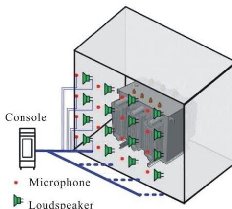
Figure 2: Schematic drawing of a planar VSB system for transformer noise control
