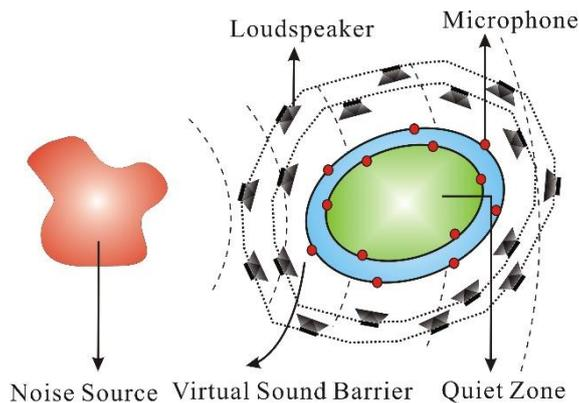
Figure 4: Schematic drawing of a double layer VSB system
