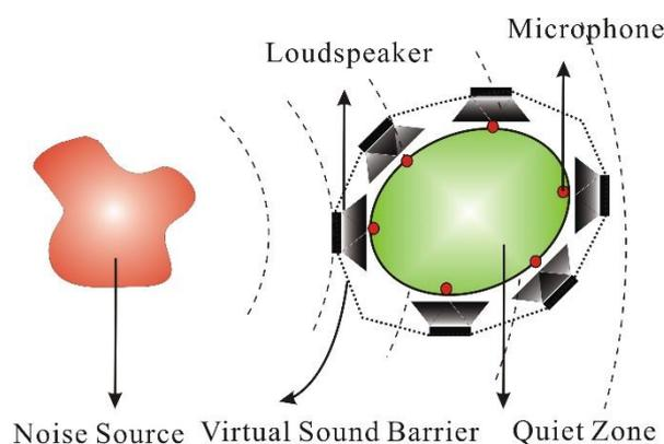
Figure 1: Schematic drawing of a VSB system
