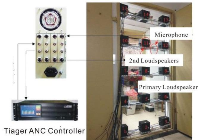
Figure 3: A photo of a planar VSB experiment system
