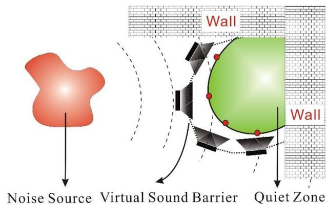
Figure 7: Schematic drawing of a corner hybrid VSB system
