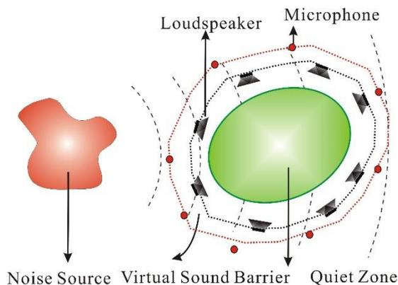
Figure 5: Schematic drawing of a mapping VSB system
