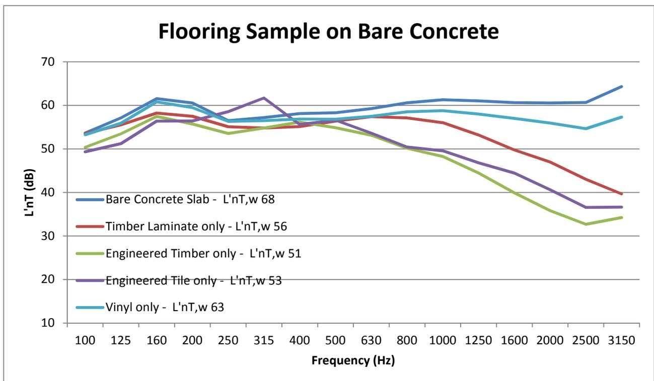
Figure 1: Flooring impact sound isolation comparison
