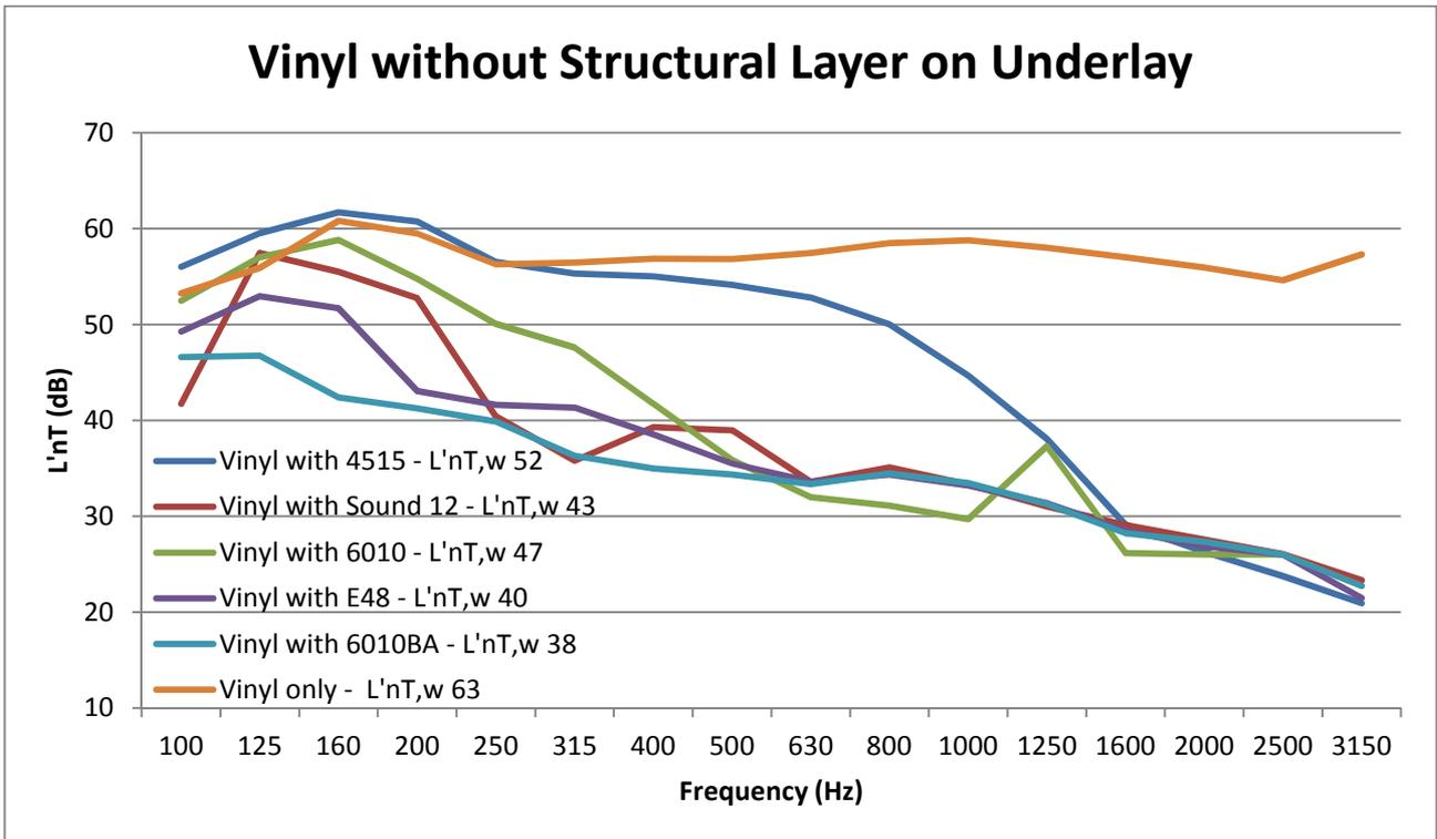
Figure 6 : Vinyl impact sound isolation without structural layer
