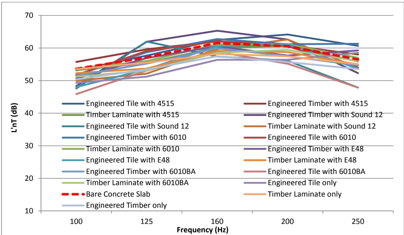
Figure 7: Comparison of low frequency performance
