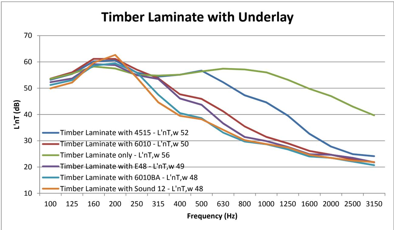
Figure 4: Timber laminate impact sound isolation
