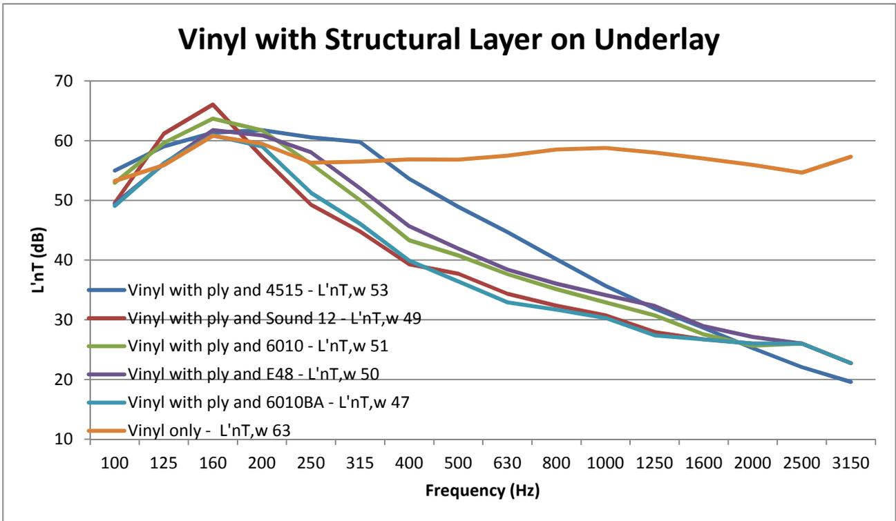
Figure 5: Vinyl impact sound isolation with structural layer
