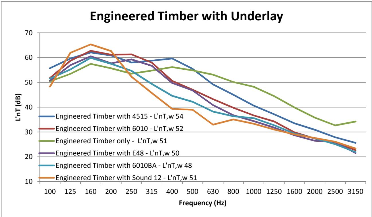
Figure 2: Engineered timber impact sound isolation
