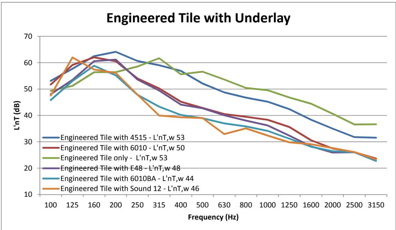
Figure 3 : Engineered tile impact sound isolation
