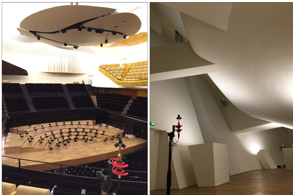
Figure 12: The tetrahedral microphone in the inner volume (left) and in the outer volume (right)
