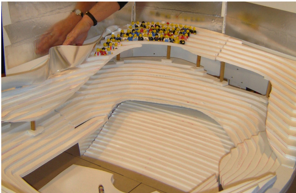
Figure 5: 1:50 Acoustic Scale Model
