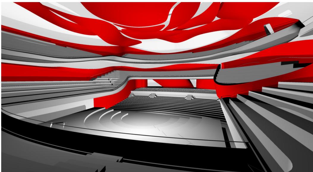
Figure 6: Rhino model with Early Reflecting Surfaces shown in Red
