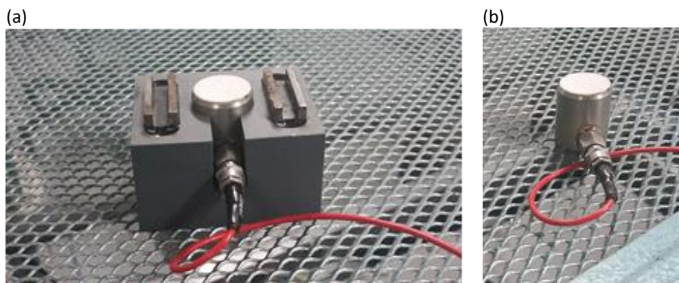
Figure 7: Sensor PAC R15 \alpha to be installed on the test rig: (a) sensor mounted in the magnetic holder, (b) sensor (the white surface is the sensor contact surface)
