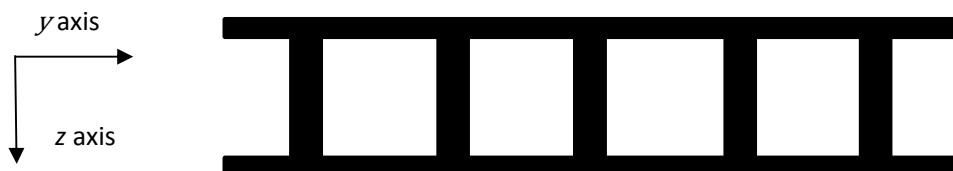
Figure 1: Cross section of double-leaf floor panel
