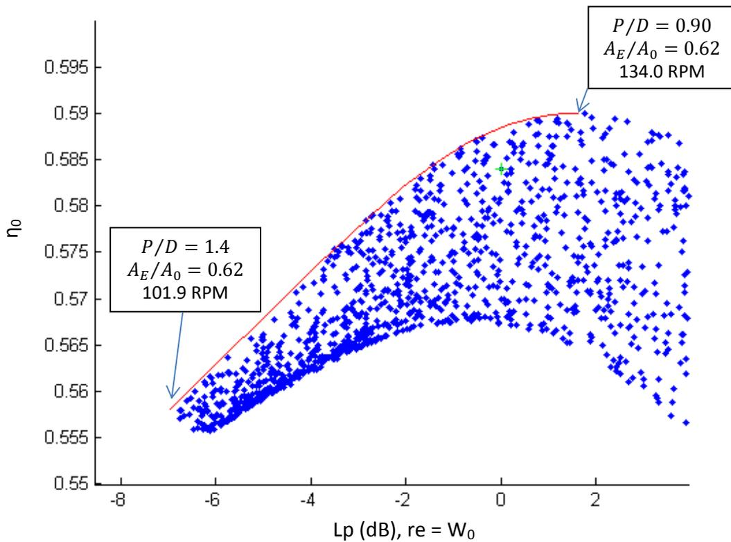
Figure 5: Efficiency against relative tip vortex noise for various 4 bladed, 2 m diameter Wageningen propellers with the Pareto-optimal front traced in red.
