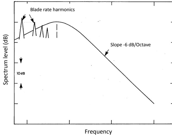
Figure 1: An example of an idealized propeller noise spectrum (Spence and Fischer, 2016)
