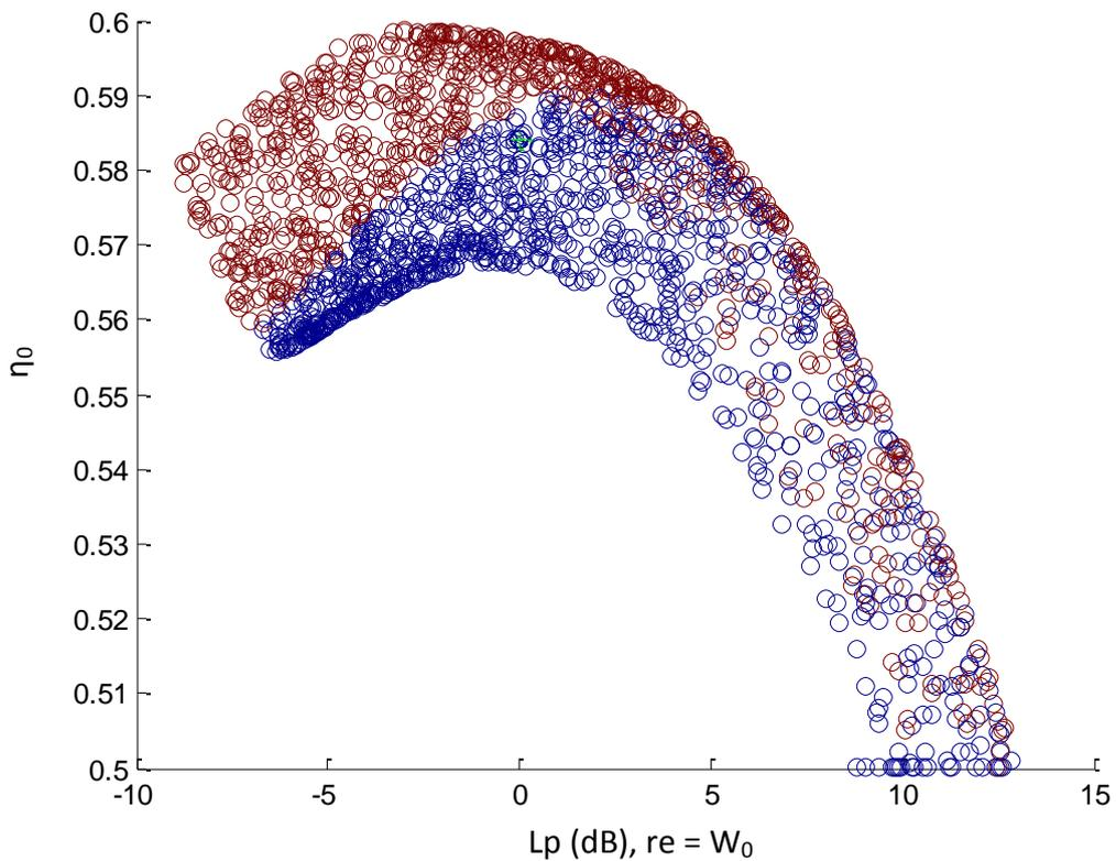
Figure 3: Efficiency against relative tip vortex noise for various 4 bladed, 2 m diameter Wageningen propellers. The red points violate the Keller cavitation criterion, the blue points do not.
