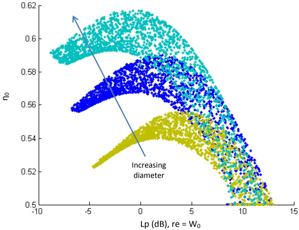
Figure 4: Efficiency against relative tip vortex noise for different diameter 4 bladed Wageningen propellers for the diameters 1.8m (mustard), 2.0m (blue) and 2.2m (teal)
