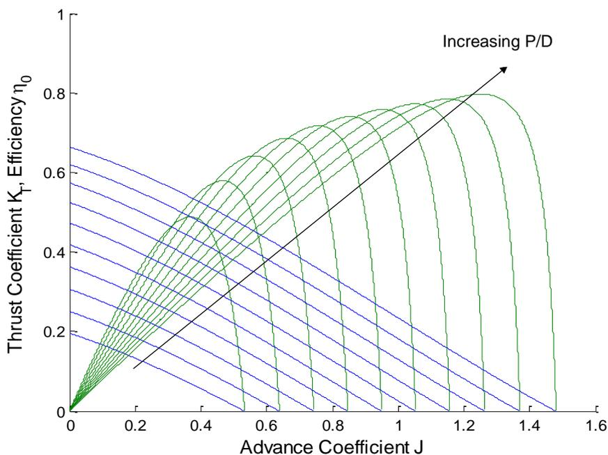
Figure 2: Thrust coefficient  $K_T$  and efficiency  $\eta$  curves for 4-bladed Wageningen B-Series propellers with blade-area ratio of 0.8 and pitch-diameter ratios ranging from 0.5 to 1.4 (Bernitsas et al. 1981).
