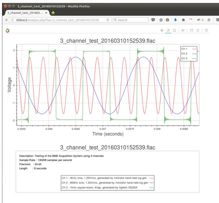
Figure 3: Screen-shot of the BBBAS web interface, showing three test signals being analysed by the device's open-source software.
