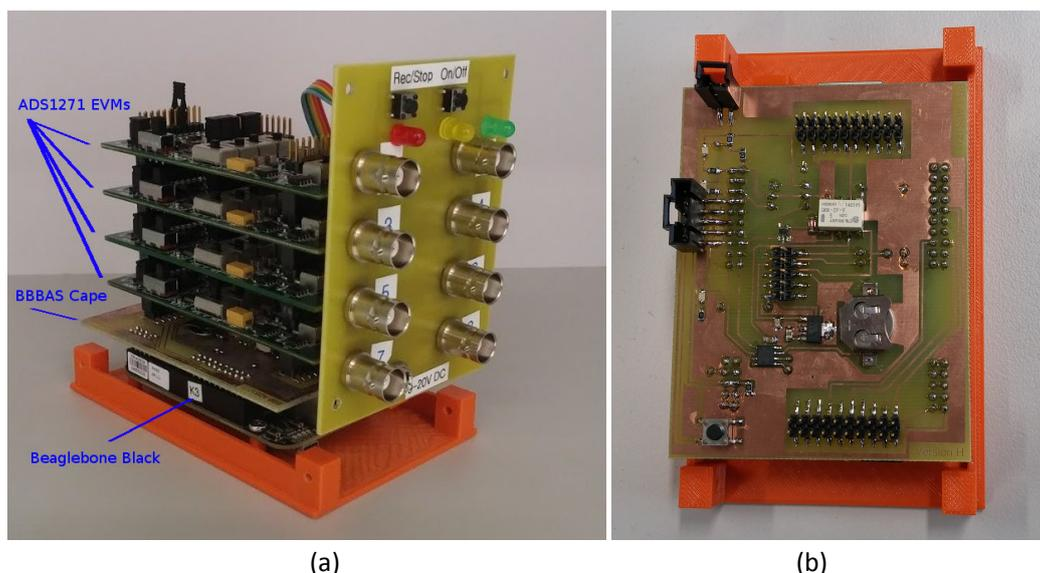
Figure 2: (a) The BBBAS without a cover, showing the ADS1271 EVM boards and the Beaglebone Black, connected via the BBBAS Cape. (b) Top view of the BBBAS Cape.
