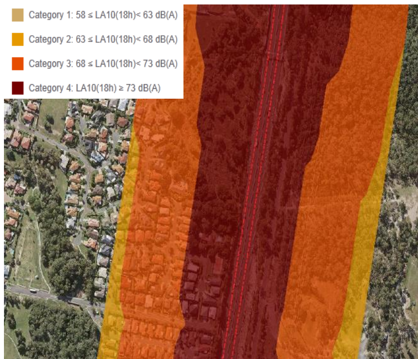
Figure 3: QDC noise contours from the first round of modelling
