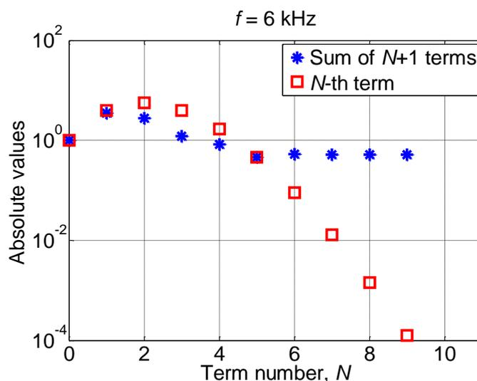
Figure 2: The absolute value of the partial sum of  $N$  terms of the series and that of the  $N$ -th term vs  $N$ . The parameters used in the calculations are:  $\Delta_c = 24.7942$  m/s,  $m = 1.17$  m<sup>-1</sup>,  $\theta_0 = 3^\circ$ .
