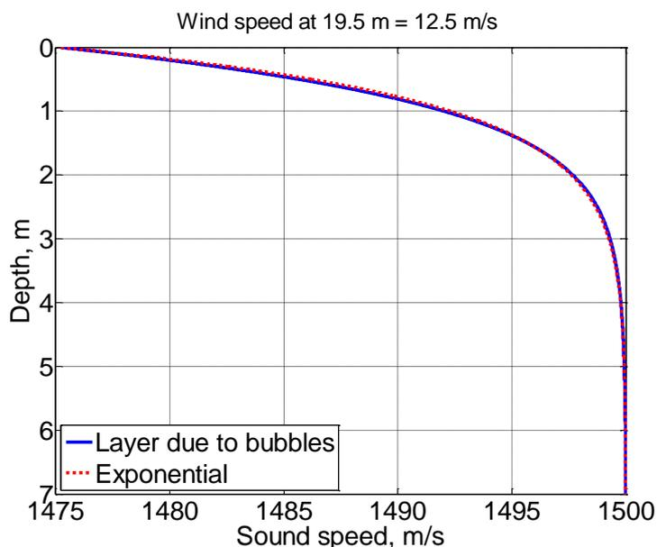
Figure 1: SSP of the surface layer due to gas bubbles compared with the “best fit” exponential SSP. Parameters used in the calculations:  $\Delta_c = 24.7942$  m/s,  $m = 1.17$  m<sup>-1</sup>.
