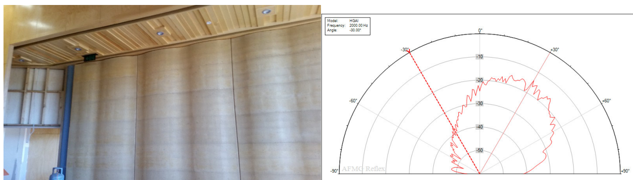
Figure 8 Side Wall Diffusion Image and Spatial Response (1 kHz)
