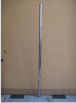
**Figure 6** Pipe bell used for a comparison study with tubular tower bell #13.
