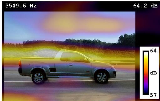
Figure 5: Beamforming data without de-dopplerization.
