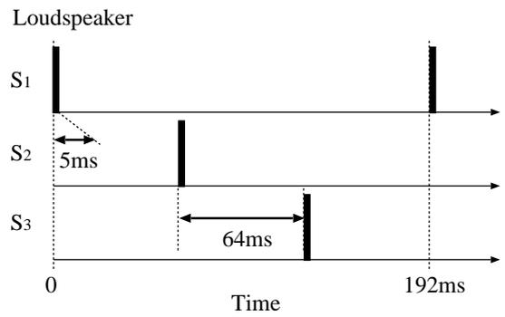
Figure 3: The emission pattern of the source signals for loudspeakers  $S_i$ . The source signals are a band-limited Gaussian noise from 18 to 24 kHz.
