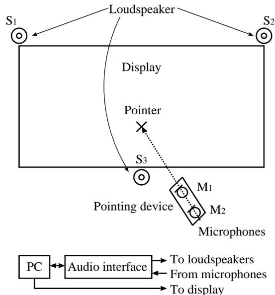
Figure 1: The configuration of our pointing system.  $S_i$  ( $i = 1, 2, 3$ ) is a loudspeaker located at known position,  $M_j$  ( $j = 1, 2$ ) is a microphone on the pointing device. The system shows the pointer that is indicated at the calculated intersection of the straight line through the estimated positions of the two microphones and the display plane.
