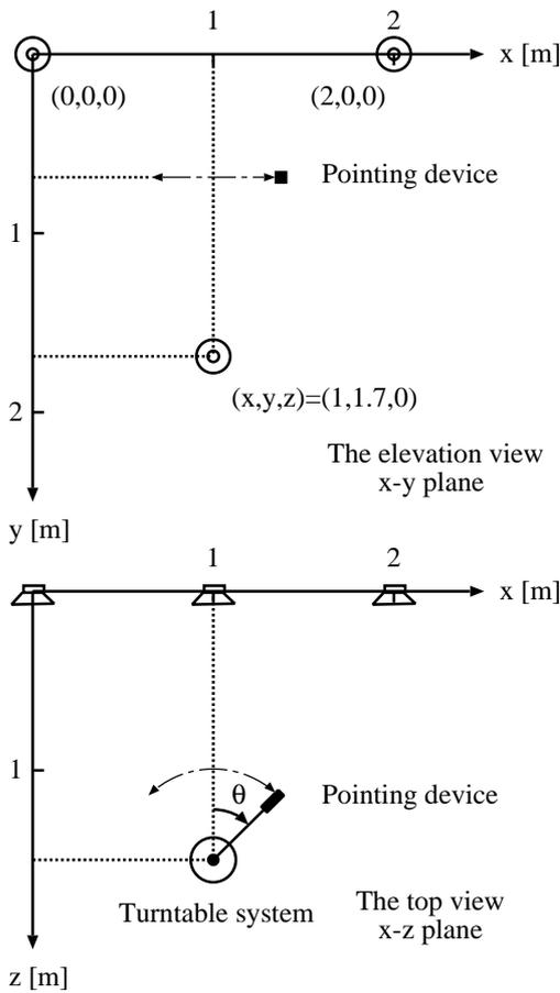
Figure 2: The experimental setup. The pointing device moves using the turntable system. The upper panel shows the elevation view and the lower panel shows the top view.
