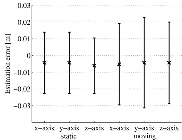
Figure 4: The estimation error of the microphones' positions. The left half shows the static case. The right half shows the moving case. The error bars show the standard deviation.
