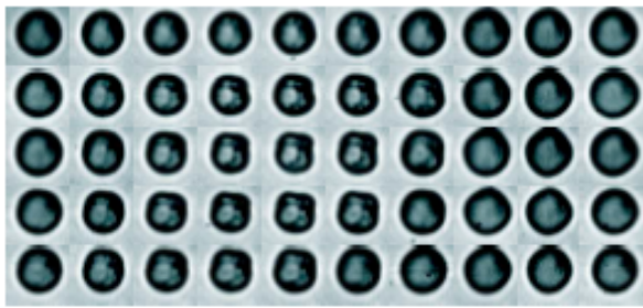
Figure 3. Optical response of an ultrasound contrast agent microbubble showing ‘compression-only’ behavior and shell buckling. ( R_0 = 3.05 \mu\text{m} , f_{drive} = 1.5 \text{ MHz} , P_a = 40 \text{ kPa} , recorded at 14.5 Mfps).
