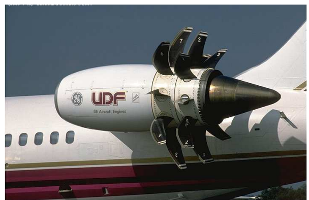
Figure 1. View of the General Electric UDF ® mounted on a McDonnell-Douglas MD-80
