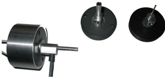
Figure 1: Different impedance probes, probe tube with an inner \varnothing = 2.5 mm mounted; probe tube with an inner \varnothing = 3.5 mm (middle), inner \varnothing = 0.8 mm (right)
