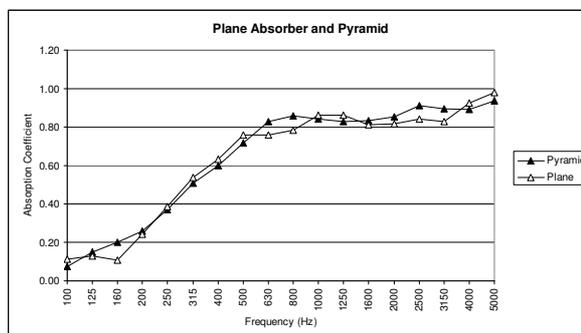
Figure 4 Comparison of plane absorber and pyramid (same volume of foam)
