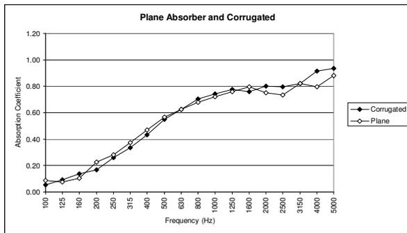
Figure 5 Comparison of plane absorber and corrugated (same volume of foam)
