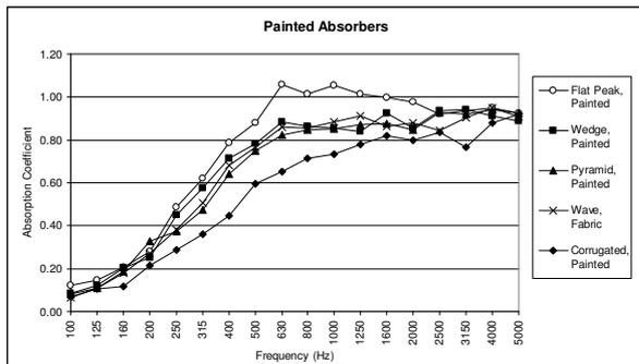
Figure 6 Effect of absorber coverings
