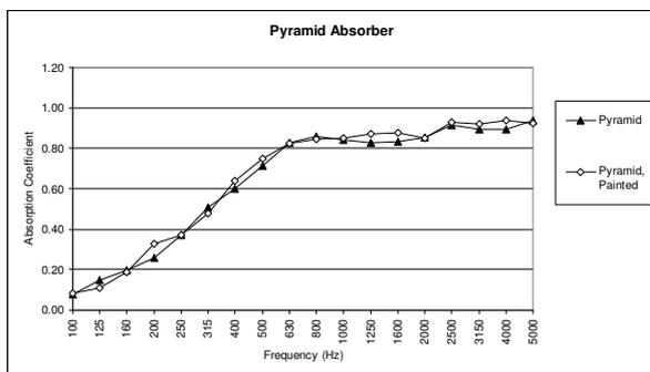
Figure 7 Effect of painting the surface of the pyramid absorber
