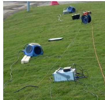
Figure 3, loudspeakers and amplifiers in place
