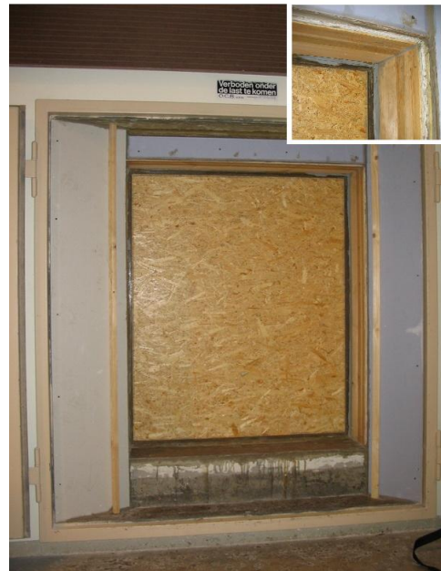
Figure 4: Measurement setup: fiberboard 9.5 mm with dimensions 1.25 \text{ m} \times 1.50 \text{ m} .
