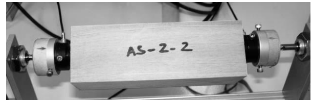
Figure 2. Transducers holding test sample
