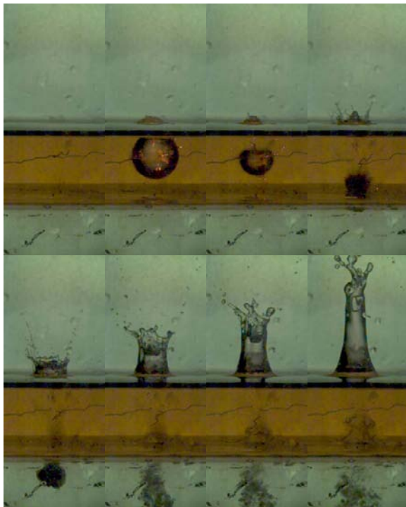
Figure 7. Three layers experiment (HFE-water-air). The layer of water is 1.8 cm high and has been colored with an orange dye. The maximum radius of the bubble is 6.1 mm. The two interfaces both exhibit an upwards jet. The frames shown correspond respectively to the times 0.0, 0.9, 1.15, 1.95, 3.15, 6, 8.9 and 17 ms.
