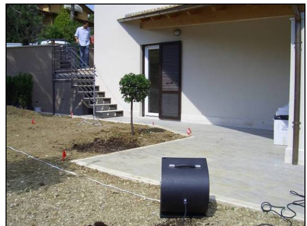
Figure 3. Case study: in situ measurement of weighted standardized sound level difference of façades D_{2m,nT,w}
