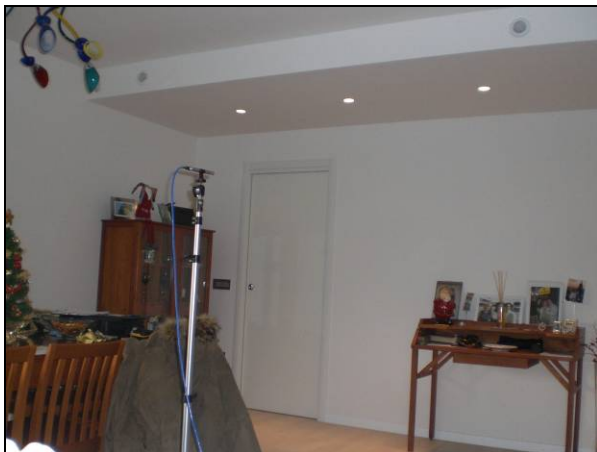
Figure 6. Case study: in situ measurement of noise level L_{Aeq} produced by CMV system into livingroom L1 (position microphone-air vents)
