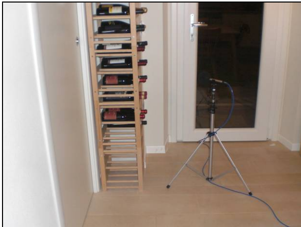
Figure 5. Case study: in situ measurement of noise level L_{ASmax} produced by wc discharge into the most disturbed room beneath (kitchen K1)
