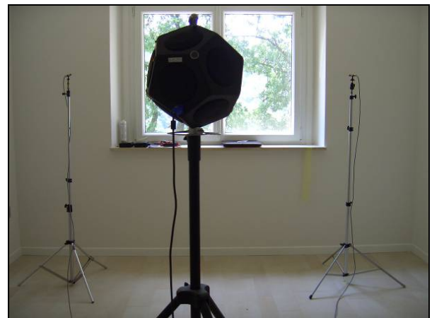
Figure 2. Case study: in situ measurement of weighted sound reduction index of partitions between rooms R'_w
