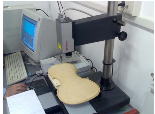
Figure 2. 3D scanner unit
