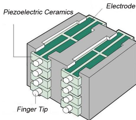
**Figure 4.** Structure of composite vibration type ultrasonic motor
