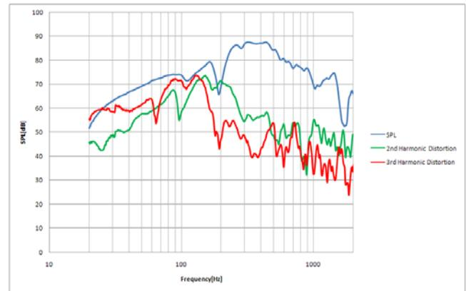
Figure12. Frequency response of the 2009 model-2
