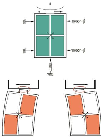
**Figure5.** Driving principle of composite vibration type ultrasonic motor
