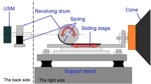
**Figure 3.** Driving principle of the loudspeaker by rotation to linear conversion mechanism
