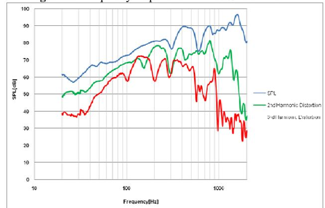
Figure13. Frequency response of the 2010 model
