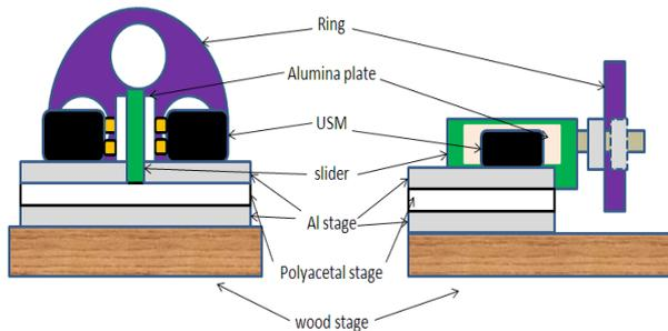
Figure11. Configuration of the 2010 Model
