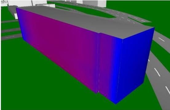
**Figure 7.** Contours of noise levels at the facade of building 1 in position A. Contours represent levels from 69 dB(A) in the purple zone to 79 dB(A) in the blue zone.
