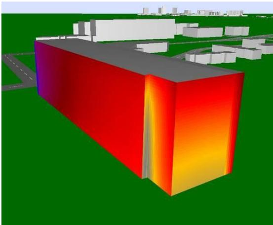
**Figure 8.** Contours of noise levels at the facade of building 1 in position A. Contours representing change in levels from 54 dB(A) in the yellow zone to 75 dB(A) in the blue zone.
