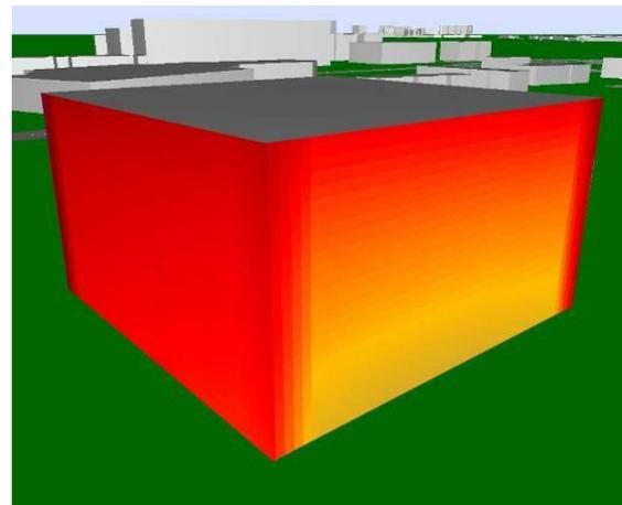
**Figure 10.** Contours of noise levels at the facade of building 2 in position A. Contours represent levels from 55 dB(A) in the purple zone to 67 dB(A) in the blue zone.
