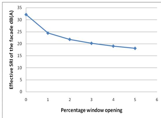
**Figure 5.** Effective SRI of the facade to traffic noise against percentage opening of the window for buildings 2 and 3.
