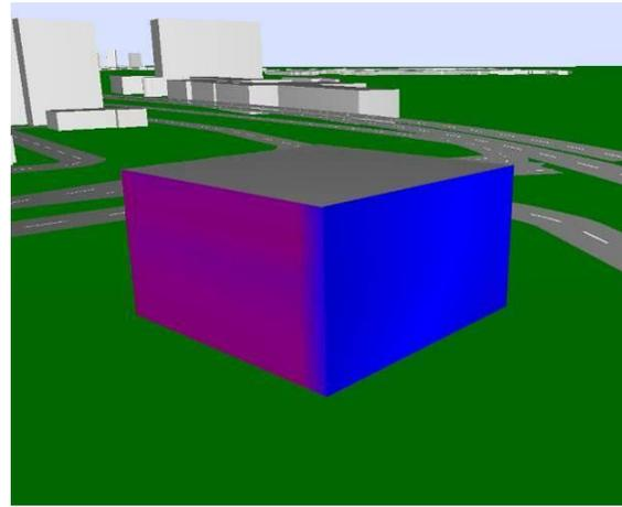
**Figure 9.** Contours of noise levels at the facade of building 2 in position A. Contours represent levels from 70 dB(A) in the purple zone to 77 dB(A) in the blue zone.
