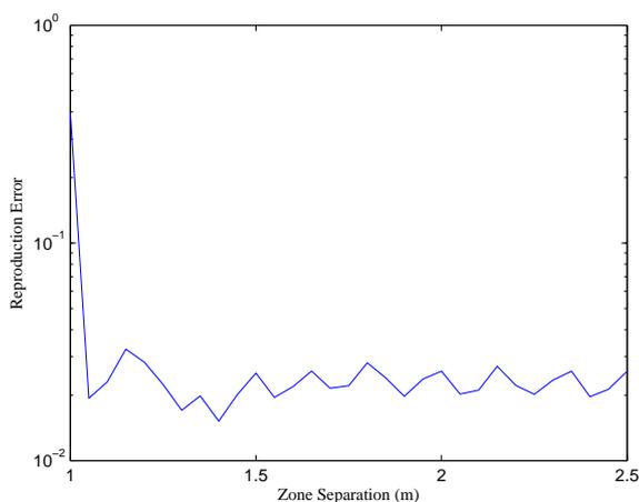
Figure 3: Reproduction error with different zone separation (in distance) for two circular reproduction zones with radius 0.4 m each using two loudspeaker array. The desired soundfields consist of 50 random plane waves at 1000 Hz. We have equally placed 17 loudspeakers on a circle of 0.4 m for each loudspeaker array.
