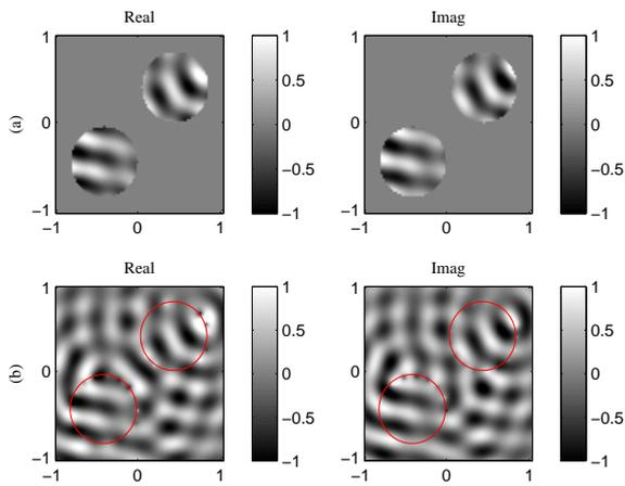
Figure 2: Reproduction of a 2D two-zone soundfield with radius 0.4 m each using two circular loudspeaker arrays. The desired soundfields consist of 50 random plane waves at 1000 Hz. Two zones are located at  $\theta^{(10)} = 135^\circ, r^{(10)} = 0.6$  m and  $\theta^{(20)} = -45^\circ, r^{(20)} = 0.6$  m respectively. (a) Desired field, and (b) reproduced field. We have equally placed 17 loudspeakers on a circle of 0.4 m for each loudspeaker array. The reproduced error in this case is 1.53%.
