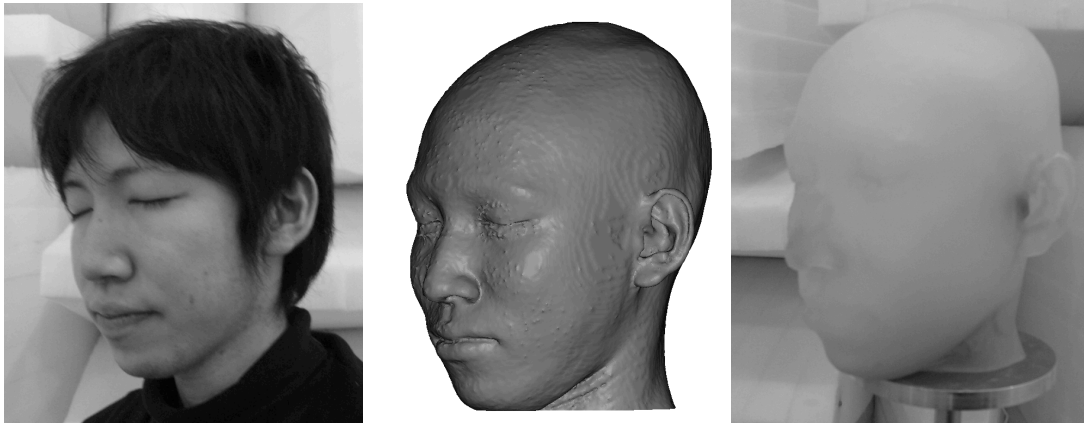
Figure 2: Comparison of an actual head (left), a three-dimensional model head (center), and a dummy-head printed using stereo lithography (right)
