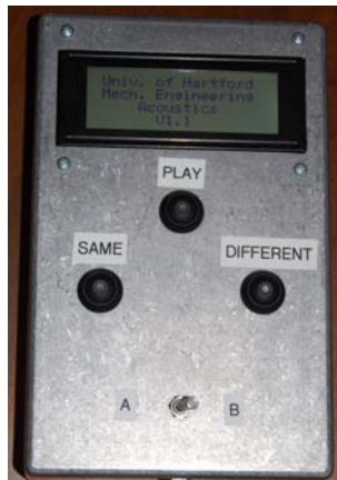
Figure 6. Custom testing box used in Study 2. Note toggle switch at the bottom of the box for the subjects to use with Test Method 2 to switch between the signals in real-time.
