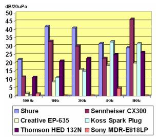
Figure 8. Sound isolation of six earphones at various frequencies at frontal incidence.
