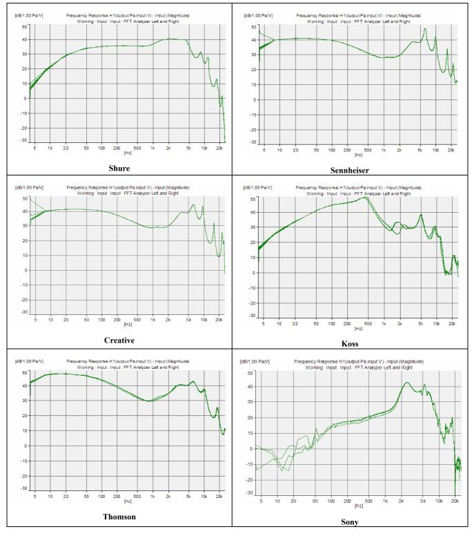
Figure 7. Transfer function measurements of six earphones.
