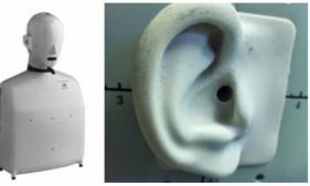
Figure 2. The BK4128 dummy-head and the DZ 9629 pinnae. Note the relatively small diameter of the (non-blocked) ear canal entrance.
