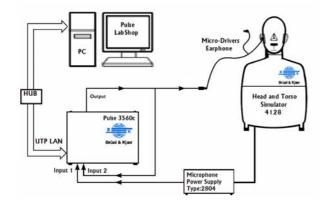
Figure 3. The measurement setup for transfer function measurements.
