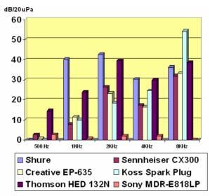
Figure 9. Sound isolation of six earphones at various frequencies at lateral incidence.
