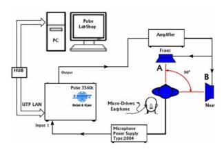
Figure 6. The measurement setup for sound isolation measurements.
