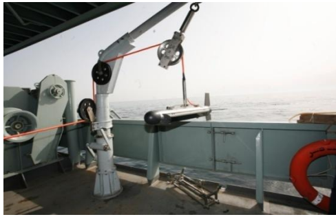
Figure 2. The towfish of the side-scan sonar
