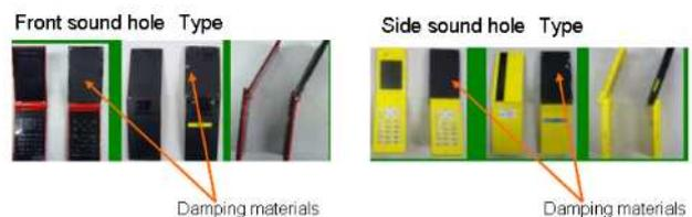
Figure 8 Mobile phones with damping materials
