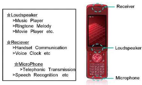
Figure 1 Acoustic devices used in mobile phones
