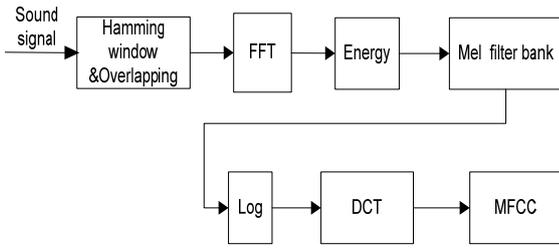
**Figure 1.** Block diagram of MFCC extraction process
