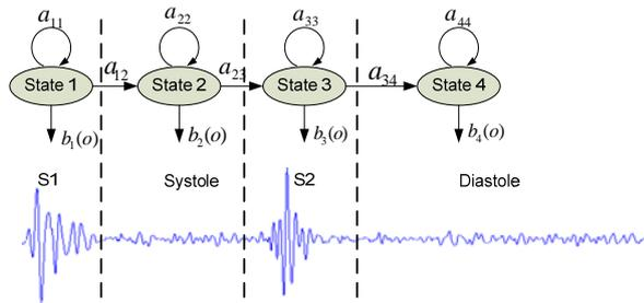
**Figure 4.** A four-state left-to-right HMM for a cycle of normal heart sound signal
