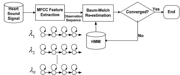
**Figure 2.** Block diagram of HMM training procedure
