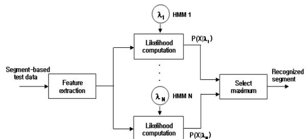
**Figure 3.** Block diagram of HMM classification procedure
