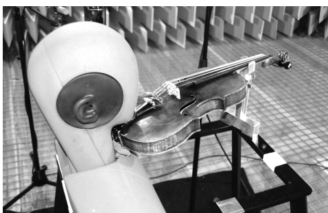
Figure 4: Dummy head microphone at the playing position in an anechoic chamber for impulse response measurements.
