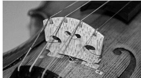
Figure 5: Bridge of the silent violin featured with piezo-electric sensors.
