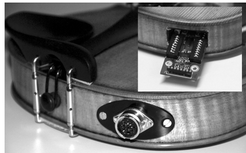
Figure 6: Phantom-powered built-in impedance converter.
