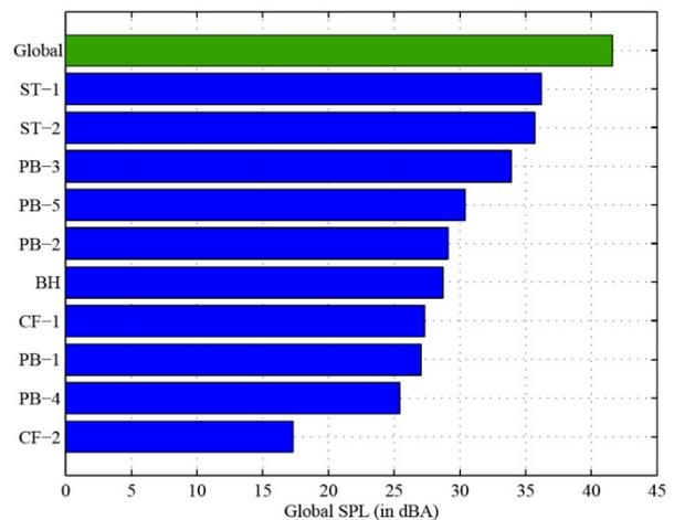
**Figure 6.** Individual noise source contributions in SPL dBA at control point receiver (blue), and overall SPL dBA (green)
