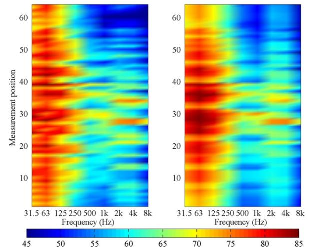
**Figure 4.** Spectrogram measured dB SPL (left) and calculated dB SPL (right)
