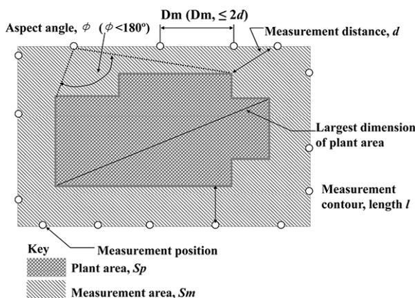
**Figure 1.** General arrangement of contour measurement positions around the plant
