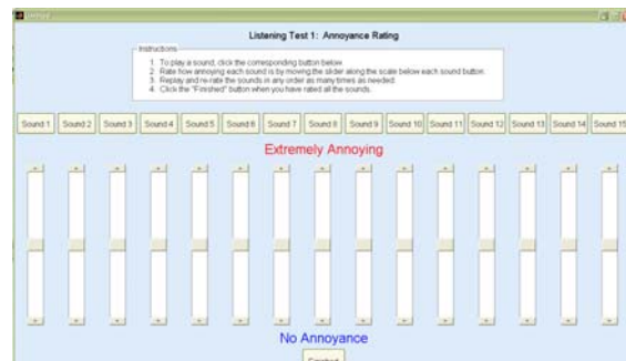
Figure 3. Computer interface for annoyance magnitude estimation experiment
