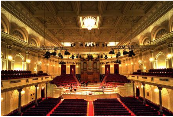
Figure 3: The Amsterdam Concertgebouw. The Concertgebouw is square in plan, and there is no stage house. The average distance from the orchestra to a listener is smaller than it is in Boston. There are no reflections from the wall behind the orchestra, as they are absorbed by the audience and the organ. The ceiling is coffered, as in Boston, and the reflections from the side walls arrive later than they do in Boston. All these factors combine to give the hall unusual clarity. The reverberation time is longer than in Boston, and the late reverberation is strong, as there are a great many surfaces that reflect the sound upward above the audience, where it can take its time to get back down. The high late reverberation level, combined with the clarity of the direct sound, give a rich sense of envelopment throughout the hall.
