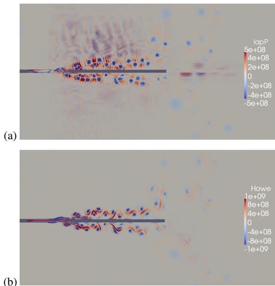
Figure 6: Spatial distributions of sound source for 2D model. (a)  $-\nabla^2 p$ . (b) Vortex sound source.
