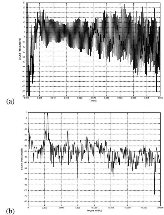
Figure 8: Sound vibration at point (D) for 2D model. (a) Acoustic pressure. (b) Power spectrum.
