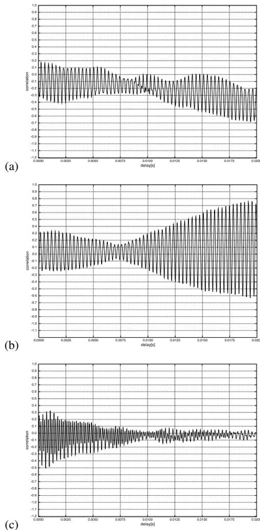
Figure 11: Correlations among dynamical variables observed at points A, B and D. (a) Lighthill at point (A) .vs. sound pressure at point (D). (b) Lighthill at point (B) .vs. sound pressure at point (D). (c) Lighthill at point (A) .vs. Lighthill at point (B).
