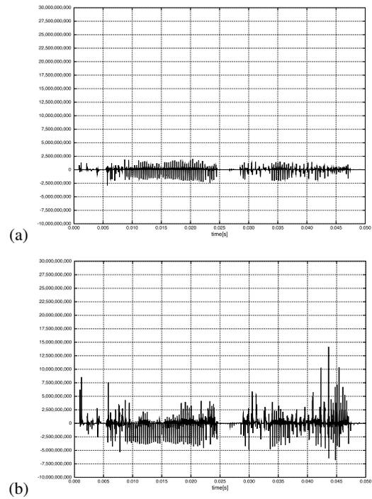
Figure 10: Sound sources at point (B) for 2D model. (a) Lighthill. (b) Howe.
