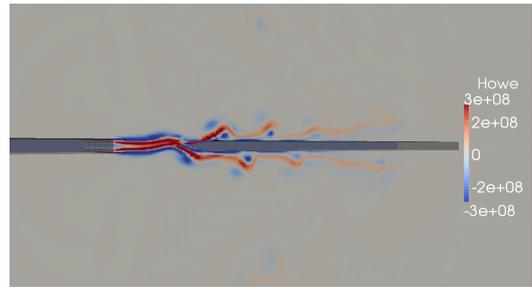
Figure 7: Spatial distribution of Vortex sound source for 3D model.
