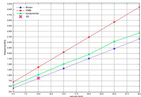
Figure 3: Jet velocity vs. frequency of acoustic vibration. Solid line: numerical result. Dotted line: Brown(eq.1). Broken line: Holger *et al.*(eq.2).
