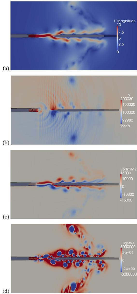
Figure 5: Spatial distributions of characteristic dynamical variables of a stable oscillation at  $V = 10\text{m/s}$  for 3D model. (a) Velocity. (b) Pressure. (c) Vorticity. (d) Lighthill’s source.
