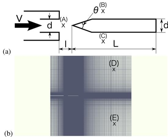
Figure 2: 2D model (a)Location of flue and edge. (b) Numerical mesh.
