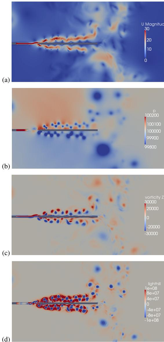
Figure 4: Spatial distributions of characteristic dynamical variables of a stable oscillation at  $V = 30\text{m/s}$  for 2D model. (a) Velocity. (b) Pressure. (c) Vorticity. (d) Lighthill’s source.
