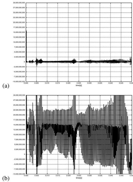
Figure 9: Sound sources at point (A) for 2D model. (a) Lighthill. (b) Howe.
