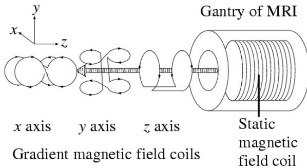
**Figure 2.** Gradient magnetic field coils in MRI equipment.
