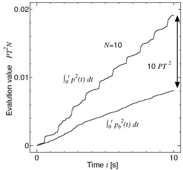
Figure 5. Technique of evaluation in equation (1) utilizing the difference value between the integral value of the signal measured including the pulse and the integral value of background noise.
