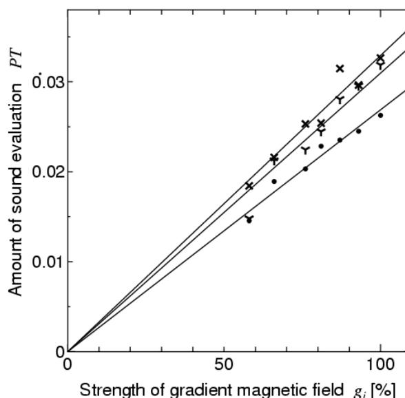
**Figure 8.** Relation between gradient magnetic field strength and amount of sound evaluation at 30cm from center (X: measurement value of x axis, Y: measurement value of y axis, •: measurement value of z axis, line: regression line).
