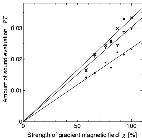
**Figure 7.** Relation between gradient magnetic field strength and amount of sound evaluation at 20cm from center (X: measurement value of x axis, Y: measurement value of y axis, •: measurement value of z axis, line: regression line).
