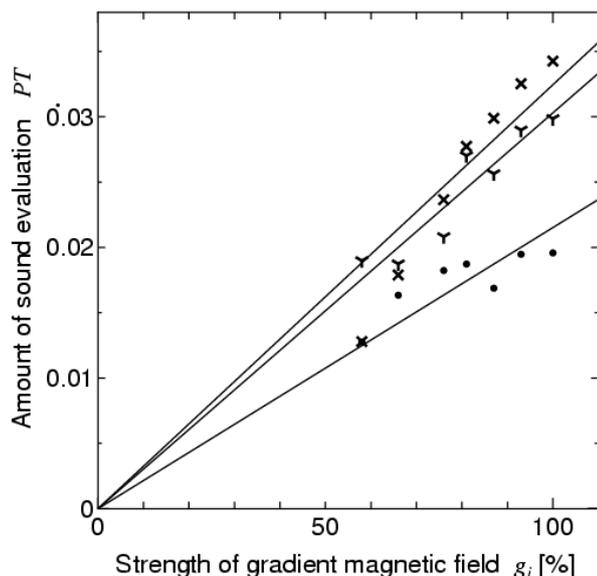
**Figure 6.** Relation between gradient magnetic field strength and amount of sound evaluation at 10cm from center (X: measurement value of x axis, Y: measurement value of y axis, •: measurement value of z axis, line: regression line).
