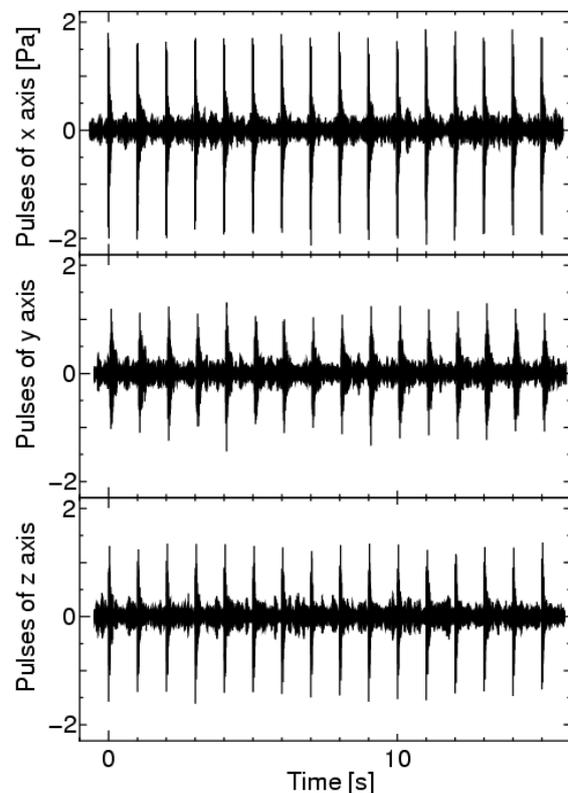
**Figure 3.** Pulses of each axes of the gradient magnetic coil driving.
