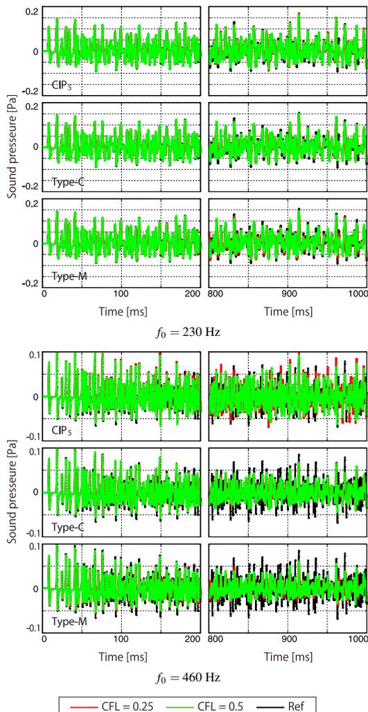
Figure 6: Numerical results in a 2-D rectangular area using CIP<sub>5</sub>, Type-C and Type-M for  $f_0 = 230$  Hz and 460 Hz.
