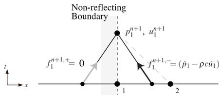
Figure 3: Example of computing boundary variables (non-reflecting).
