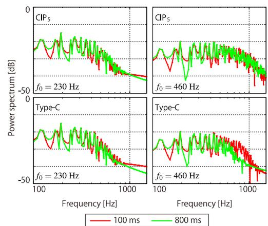
Figure 8: Comparison of power spectrum at  $t = 100$  ms and 1000 ms: The FFT length is 2048 points.
