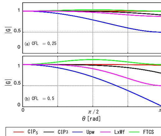
Figure 4: Comparison of numerical stabilities of CIP<sub>5</sub>, CIP<sub>3</sub>, 1st up-wind (Upw), Lax-Wendrof (LxWf) and 2nd FTCS schemes by using the von Neumann method.  $G$  is the amplification factor and  $\theta$  is the phase angle. (a) CFL = 0.25, (b) CFL = 0.5.
