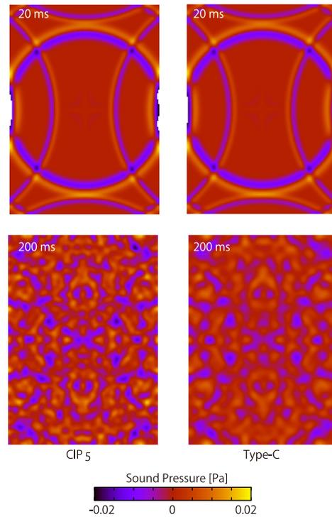
Figure 10: Contour maps of sound pressure in the  $xy$ -plane calculated using the CIP<sub>5</sub> and Type-C methods.
