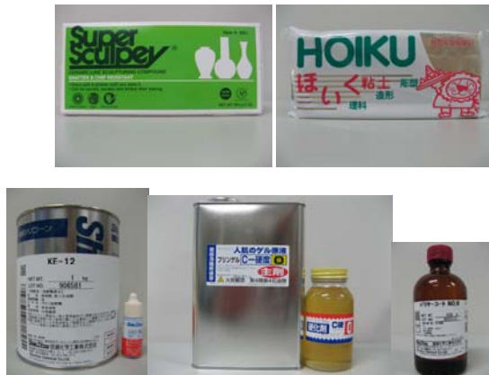
Figure 6. Materials used for the molding the tongue figure models. Ceramic-like sculpturing compound, Oil clay, Silicon, urethan gel, and barrier coating liquid.
