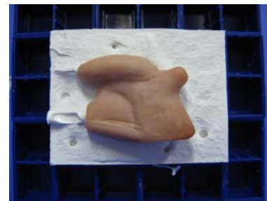
Figure 10. The upper half of the mold was made.
