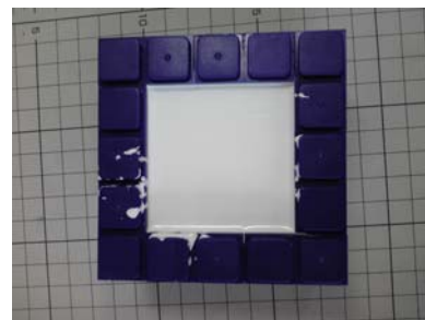
Figure 9. Sillicone was poured to the upper half of the model.
