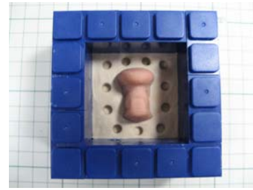
Figure 8. The bottom half of the original model was sinked in oil clay in the frame. Dwelling holes were made using a stick.
