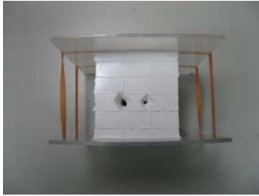
Figure 11. Upper and lower halves of the mold was tightly put together. One hole is for pouring urethan rubber gel and the other one is for removing air.
