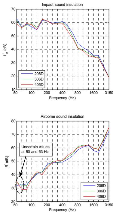
**Figure 12.** In-situ measurements of impact and airborne sound insulation in 1/3 octave bands
