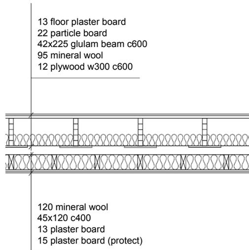
**Figure 1.** Separate floor and ceiling in a volume construction
