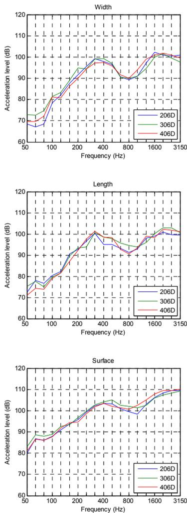
**Figure 10.** Vibrations in a completed volume with parquet floor, ready for shipping
