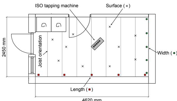
**Figure 2.** The measurement setup and definition of terms
