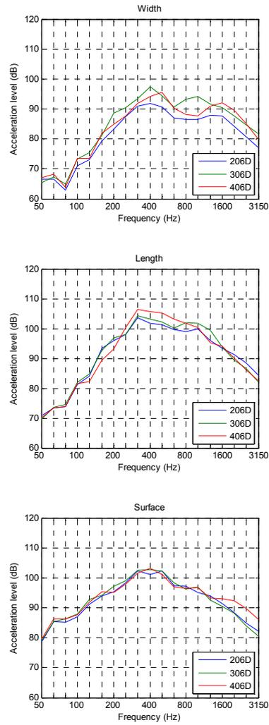
**Figure 9.** Vibrations with a small patch of parquet placed under the ISO tapping machine on the gypsum floor in a volume
