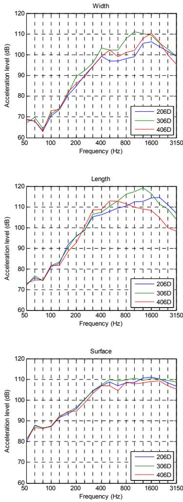
**Figure 8.** Vibrations on a floor with gypsum boards where the walls and ceiling have been attached to form a volume
