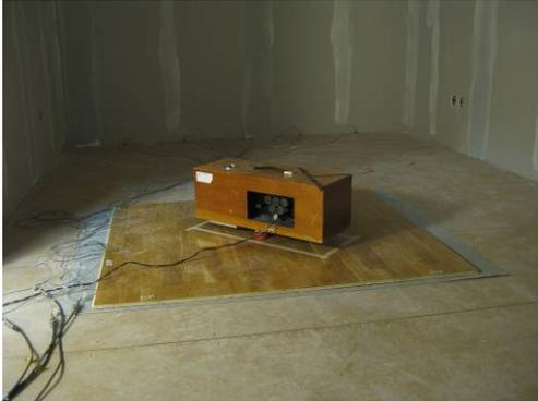
**Figure 5.** A 1 m<sup>2</sup> square patch of parquet was placed beneath the ISO tapping machine inside the volume
