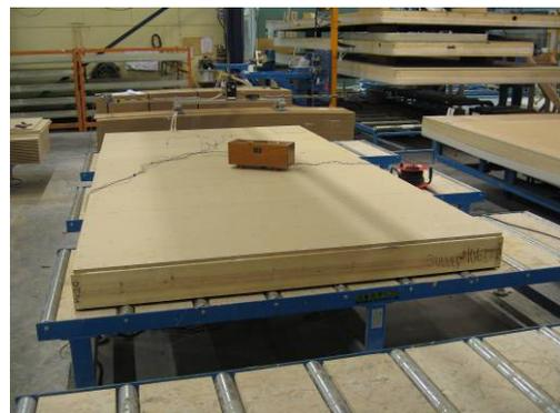
**Figure 3.** The simple floors with plates on beams were measured in the production line, on tables with rollers
