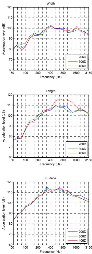
**Figure 6.** Vibrations on a floor consisting of wooden plates on beams
