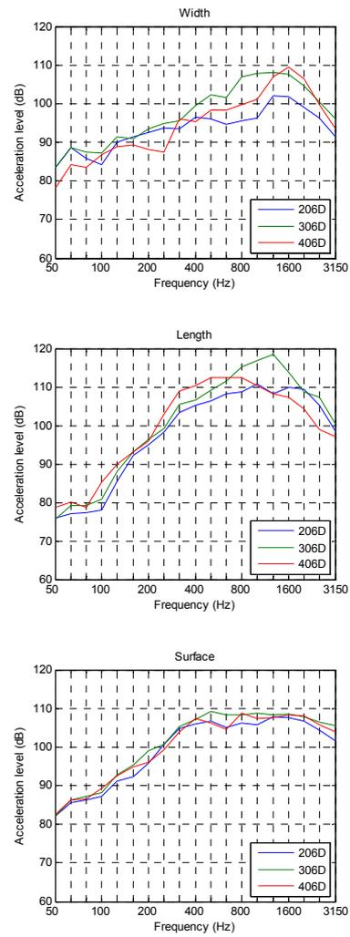
**Figure 7.** Vibrations on a floor element with glued gypsum boards
