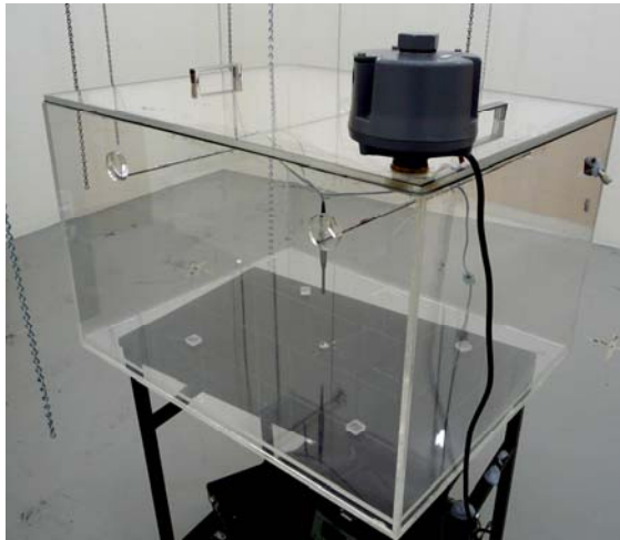
Figure 1. Rectangular Perspex room (793 x 638 x 494) mm
