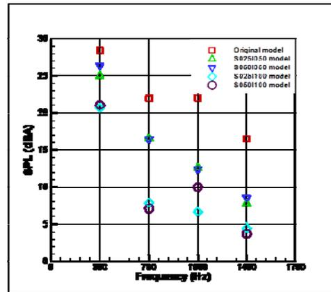
Figure 8. Prediction of low-noise centrifugal fan designs
