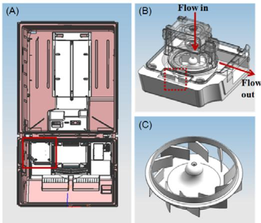
**Figure 1.** CAD data of the targeted refrigerator: (A) installation position of the targeted fan, (B) the targeted fan system, and (C) the targeted centrifugal fan
