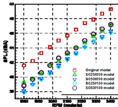
**Figure 11.** Measure overall SPLs of fans according to its rotating speeds.
