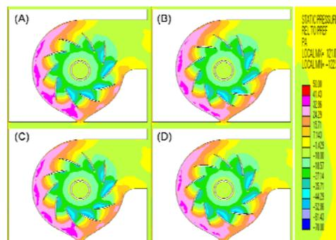
**Figure 3.** Static pressure contour at the middle cross-section in the span-direction of fan blade: at (A) beginning, (B) 1/4, (C) 1/2, and (D) 3/4 of the period of the blade passing frequency
