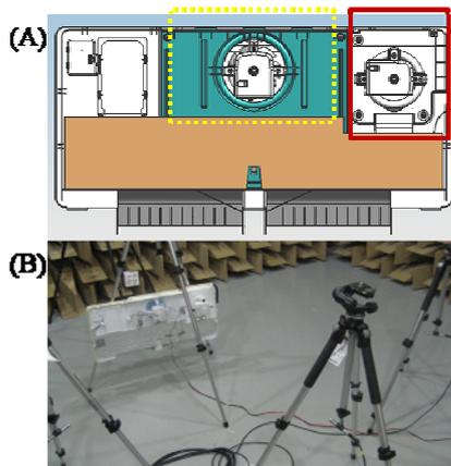
**Figure 10.** Fan assembly and experimental set up: (A) CAD data of fan system assembly and (B) experimental set up
