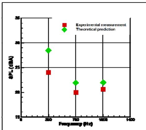
**Figure 5.** Comparison of the BPF noise levels between prediction and measurement
