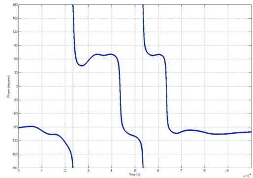
**Figure 11.** The decoded PSK acoustic communications signal [1 1 0 0 1 0 1 1 1 1]
