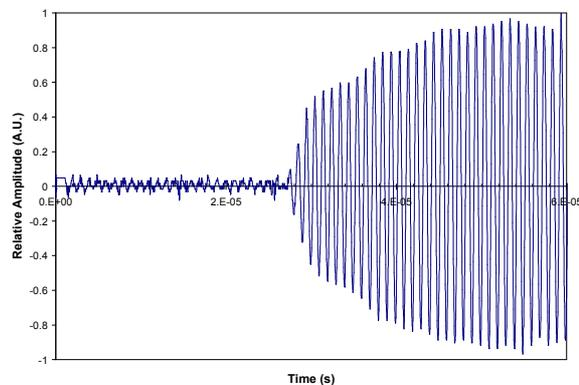
**Figure 7.** The transient response of the acoustic communications channel showing the rise time
