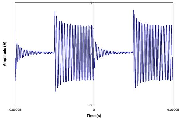
**Figure 8.** The transmitted ASK (OOK) acoustic communications signal
