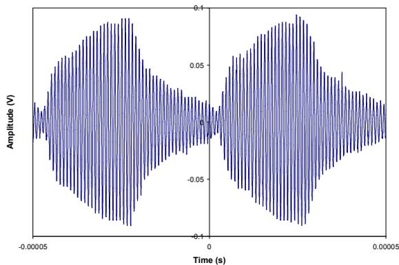
**Figure 9.** The received ASK (OOK) acoustic communications signal
