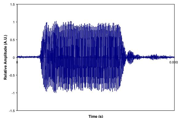
**Figure 6.** The transient response of the acoustic communications channel to an input tone burst
