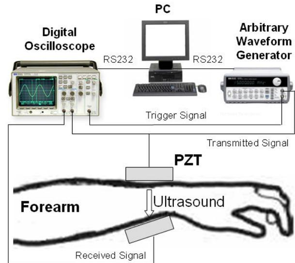
Figure 2. The setup of the acoustic-transmissions channel
