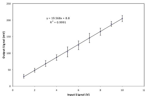
**Figure 4.** The transfer function of the acoustic communications channel at resonance
