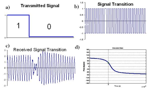
**Figure 1.** The PSK communications encoding and decoding; a) The initial digital information, b) the phase encoded signal, c) the received signal, and d) the recovered phase information
