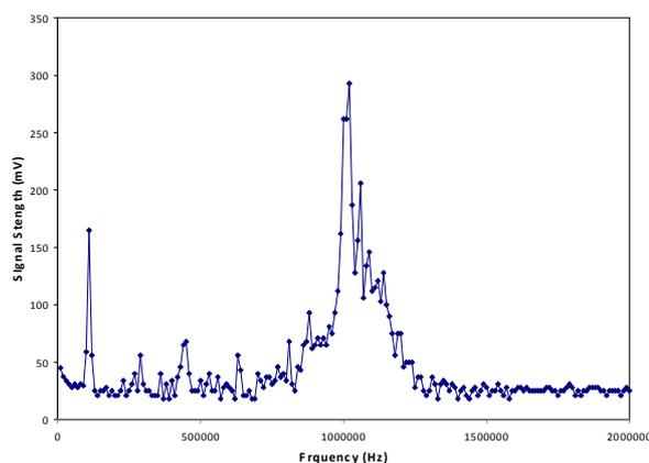
**Figure 5.** The frequency response of the acoustic communications channel
