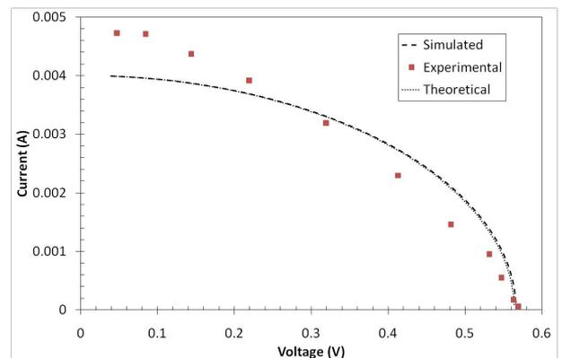
**Figure 13.** Load current as a function of the voltage, IV curve
