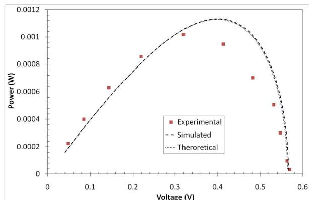
**Figure 14.** Power delivered to the load as a function of the voltage, PV curve
