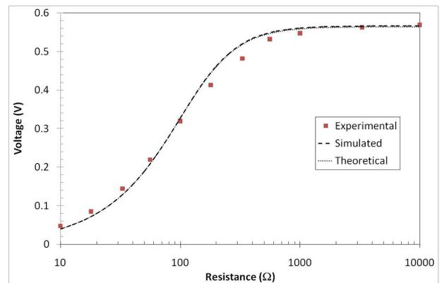
**Figure 12.** Voltage as a function of load resistance for the power harvesting
