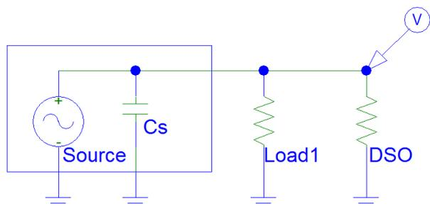
**Figure 3.** The PSpice simulation circuit, with the AC current source and the source capacitor as the piezoelectric receiver in parallel with the Load and DSO
