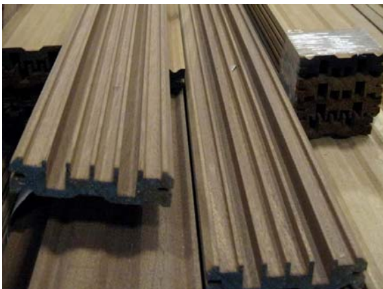
Figure 6 Example of a low profile milled QRD timber paneling suitable for small music rooms but has limited diffusion frequency range.
