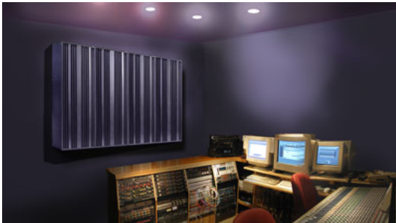
Figure 5 Example of a QRD panel installed in a sound control room. (The QRD panel shown is the 200mm deep commercially available PrimaAcoustic 'Razorblade Quadratic Diffuser' effective from 400Hz and upwards.)
