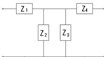
**Figure 5** One section of the equivalent electrical circuit model of the tube.
