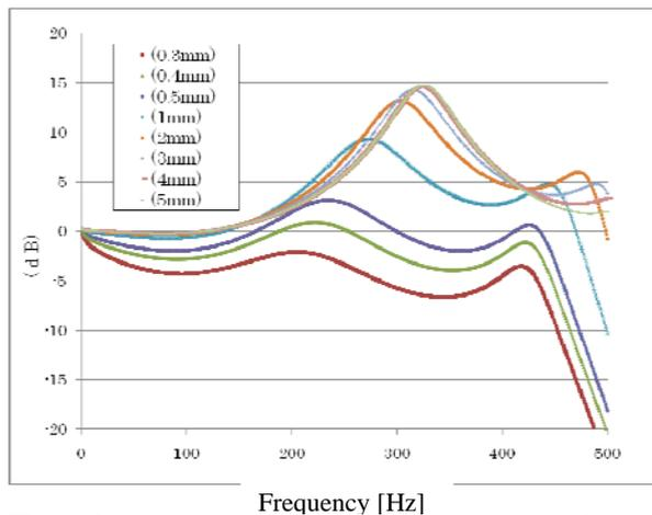
Figure 9 Frequency characteristics 0Hz to 500 Hz of voiced consonant /b/ in the case that wide length of the velum is changed 0.3 mm to 5 mm.
