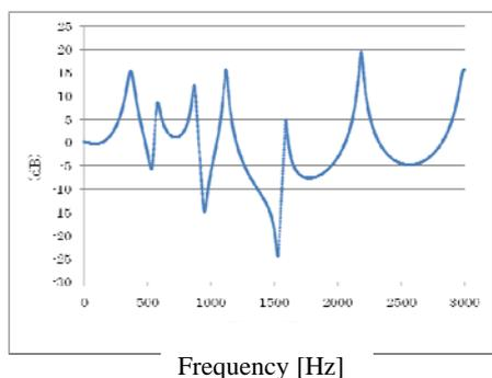
Figure 7 Frequency characteristics of consonant /m/.
