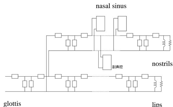
**Figure 6** The equivalent electrical circuit model of the vocal tract.
