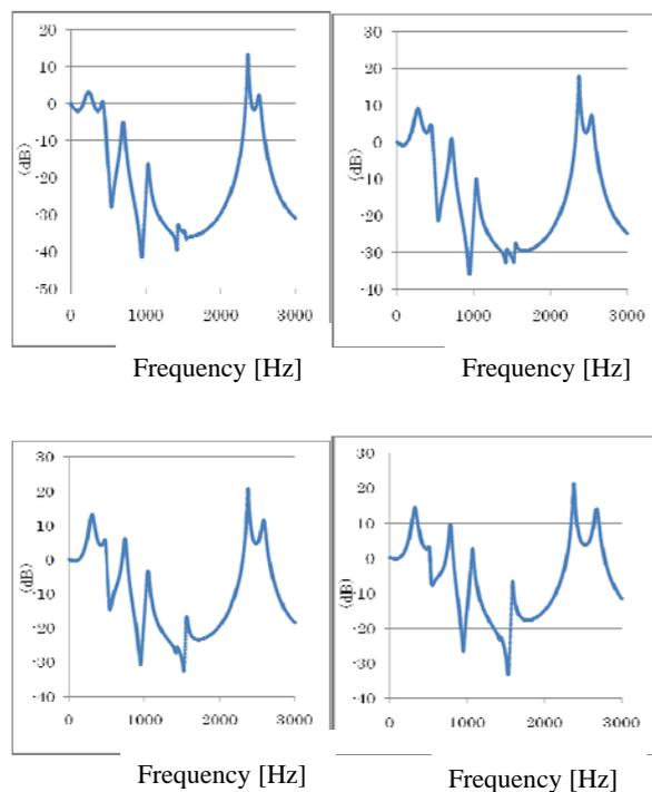
Figure 8 Frequency characteristics of buzz of voiced consonant /b/ in the case that widths of the velum are changed 0.5 mm(upper, left), 1 mm(upper, right), 2 mm(lower, left), and 4 mm(lower, right).
