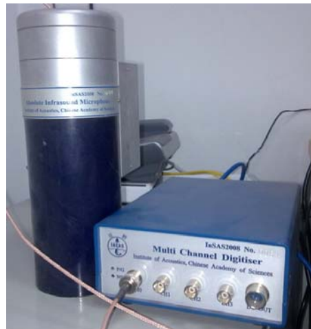
Figure 2. InSYS 2008 Infrasound microphone and network transmission device
