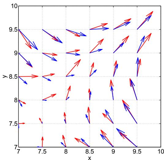
Figure 4: Reverberant intensity vector distribution over the horizontal plane in a cubic room  $10 \times 10 \times 10 \text{ m}^3$  with  $\alpha = 0.1$  and diffuse reflecting boundaries. Particle-tracing simulation (red arrows) and diffusion theory (blue arrows).
