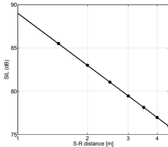
Figure 5: Total sound intensity level (SIL), including both direct and reverberant field, as a function of the source distance inside a sphere with radius  $R = 5 \text{ m}$  and  $\alpha = 0.1$ : diffusion theory (●), theoretical value of the direct field (solid line)
