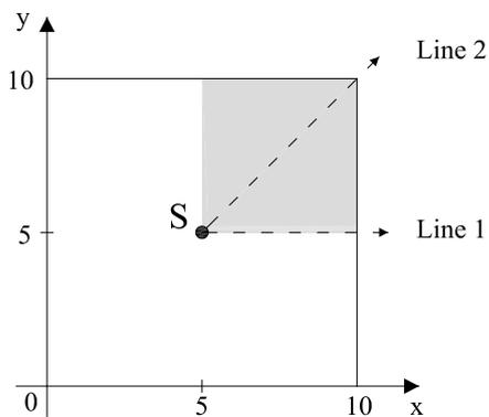
Figure 1: Upper view of the  $10 \times 10 \times 10$  m<sup>3</sup> cubic-room case study with the source position  $S$  and the two dashed lines along which sound pressure and intensity levels are evaluated.
