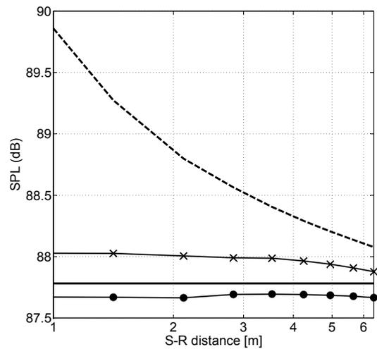
Figure 2: Sound pressure level (SPL) of the reverberant field inside a  $10 \times 10 \times 10$  m<sup>3</sup> cubic room with  $\alpha = 0.1$  and diffuse reflecting boundaries. The results are plotted along Line 2: particle-tracing simulation ( $\times$ ), Sabine's statistical theory (solid line); (- -) and ( $\bullet$ ) indicate respectively the SPL calculated with the diffusion model from  $w(\mathbf{r})$  and  $w_c(\mathbf{r})$ .
