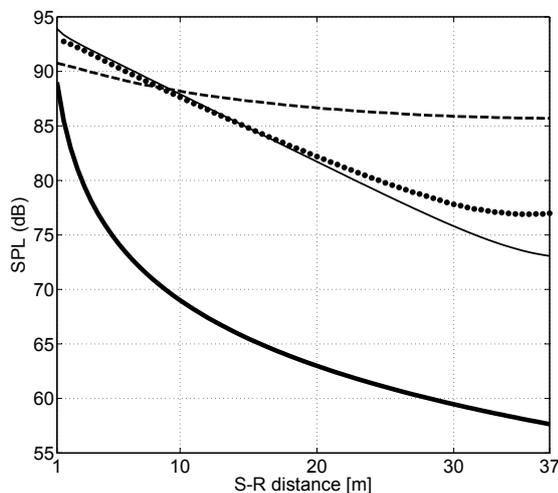
Figure 6: Sound pressure level (SPL) of the sound field inside a  $4 \times 4 \times 40 \text{ m}^3$  long room with  $\alpha = 0.1$ , as a function of the source-receiver distance (S-R distance): diffusion theory (thin solid line), particle-tracing simulations for the room with diffuse (•) and specular (- -) boundaries, direct field (thick solid line).
