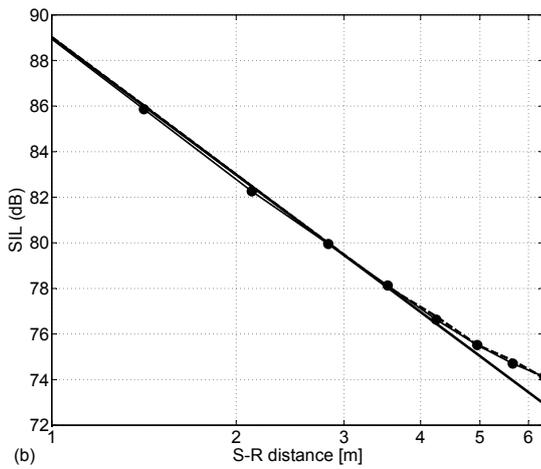
Figure 3: Total sound intensity level (SIL) as a function of the source-receiver (S-R) distance, including both direct and reverberant field, inside a  $10 \times 10 \times 10 \text{ m}^3$  cubic room with  $\alpha = 0.1$ . Results plotted along Line 1 (a) and Line 2 (b): particle-tracing simulation (- -), diffusion theory (●), theoretical value of the direct field (solid line)
