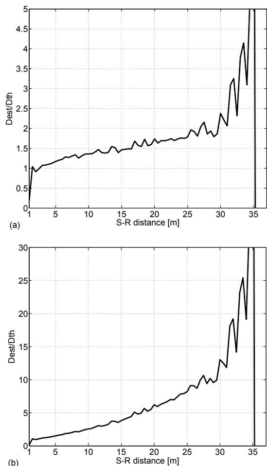
Figure 8: Ratio between the estimated and the theoretical diffusion coefficient inside a  $4 \times 4 \times 40 \text{ m}^3$  long room with  $\alpha = 0.1$  and diffuse (a) or specular reflecting boundaries (b).
