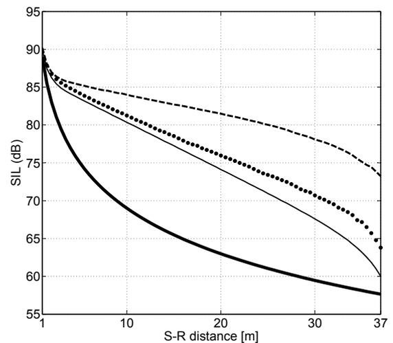
Figure 7: Sound intensity level (SIL) of the sound field inside a  $4 \times 4 \times 40 \text{ m}^3$  long room with  $\alpha = 0.1$ : diffusion theory (thin solid line), particle-tracing simulations for the room with diffuse (•) and specular (- -) boundaries, direct field (thick solid line).
