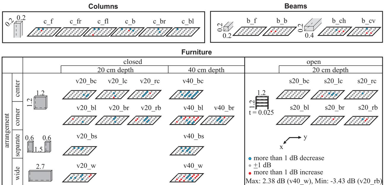
Figure 5—Differences from the normal model in  $SD_f$  at 25 receiving points in the listening area.
