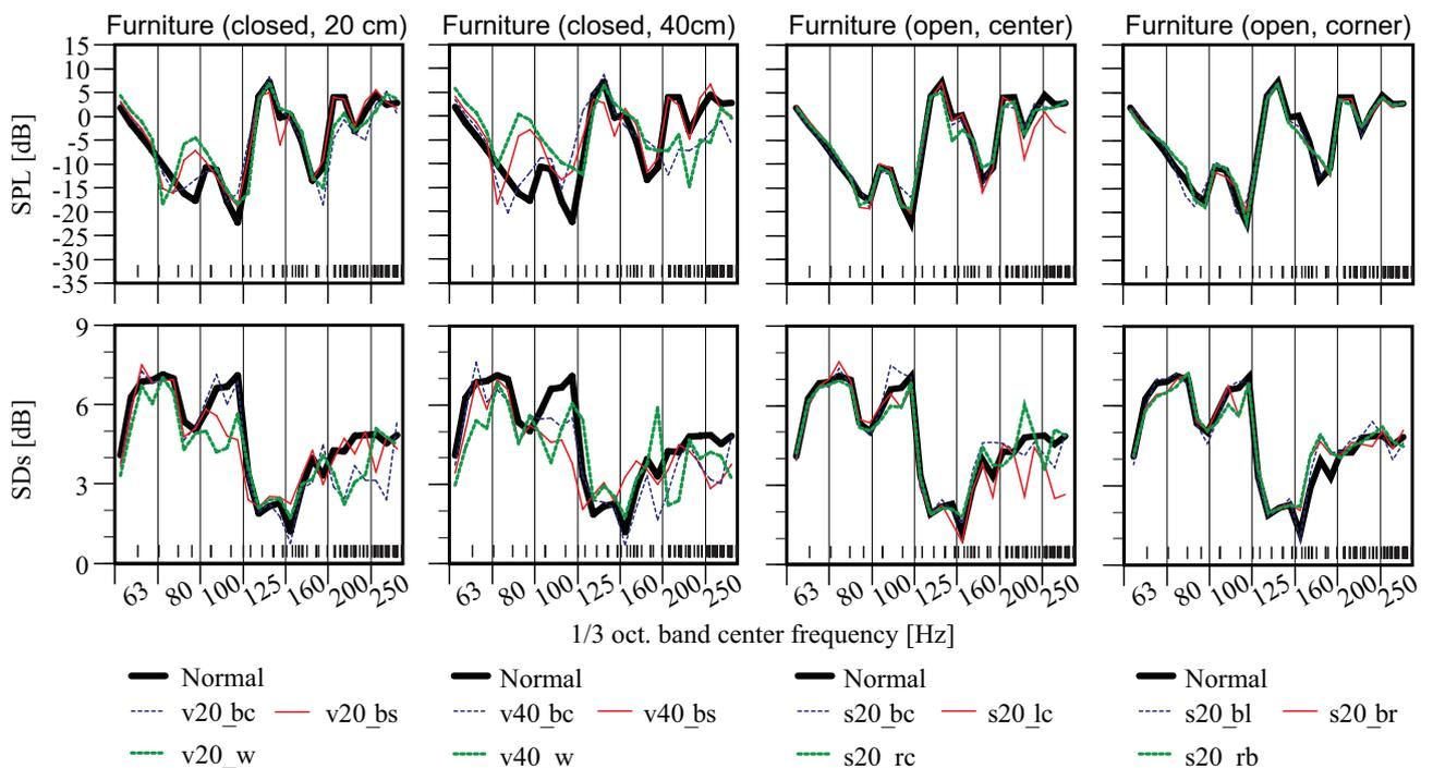
Figure 3—Frequency responses at R, and  $SD_s$  in the listening area. Eigenfrequencies are calculated from room size ratio of the normal model.
